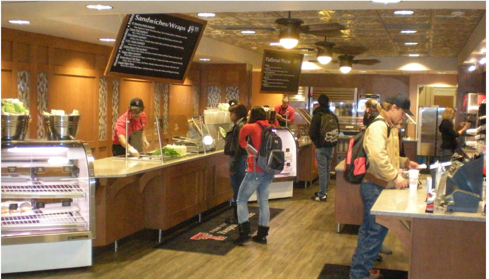
Essence™ counters shown with solid surface tops and Versa-Gard® Euro-style vertical glass food shields. Counter fronts are real wood panels applied in the field by a millwork contractor to match the interior theme of the space.
